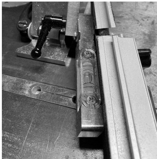
Figure 6 Setting up the miter fence with the JS3
